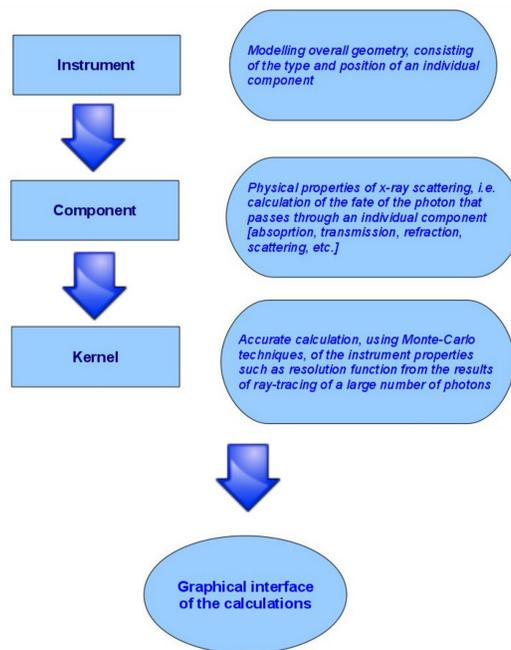
Figure 1: Three levels of the code structure.
